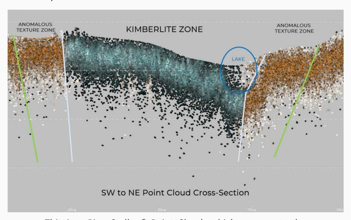
This is a Pipe Stalker® Point Cloud, which represents the subsurface, in 3D. This illustrates Pipe Stalker® capacity to differentiate four subsurface variables: differences in densities; differences in textures; differences in resistivities and structural bounds. In this case, anomalous texture zones were identified and the kimberlite zone was selected, with distinct structural bounds, even under water.
